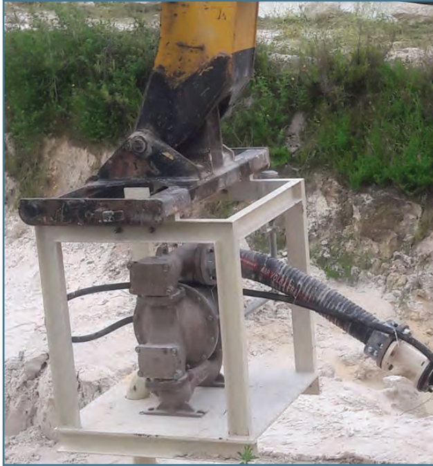
MISTRAL pump 4" for silice extraction (Italy)
